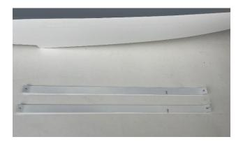
Take the other joiner struts and in one of the ends insert a 4mm x 20mm hex head bolt and flat washer and place in the joiner hole. Then take any of the two rear cross struts and insert the bolt through the bent end that has a shallower angle of the strut. Drive through the float "ear" hole with bolt, and screw to the main rear strut. Do not fully tight the bolt.
