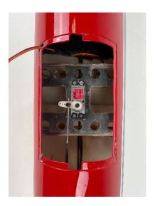
Make a slot as show in the picture below to allow the servo extension to pass through. Complete this section by closing the servo by with the cover supplied. Use a good quality clear tape. If you are super confident on your servo and installation you can apply clear silicone.
