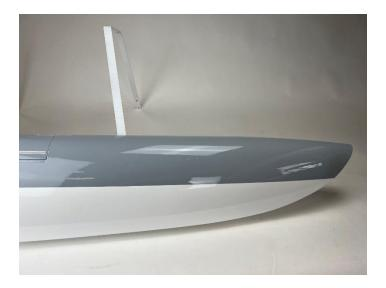
Place the two floats on a flat table and separate each other as they were on the airplane. Each float has two "ears" where the struts are attached. Push the strut thru the float slot. The main strut has a notch that must align with the inside float structure. Install the front and rear main struts.
